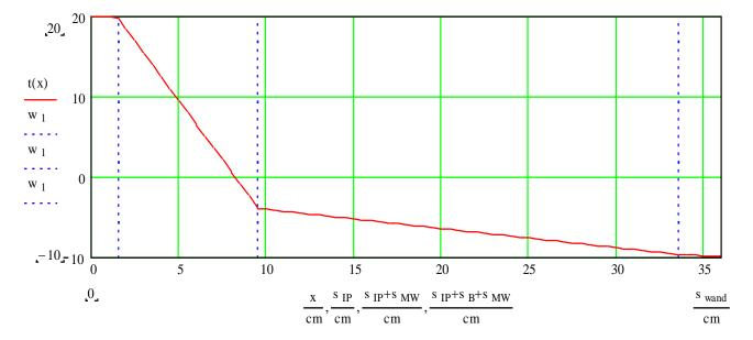
As sketched in both diagrams, the largest temperature drop is across the insulating layer even though the brick layer is much thicker!
